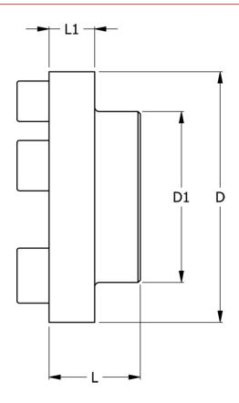
D = 110 D1 = 86 L = 40 L1 = 14 Max bore = 48 Torque (N m) = 160
